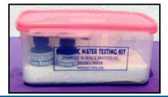
The kits are compact, portable and can test 40 samples of water. Tests for specific parameters can be added at user's request
